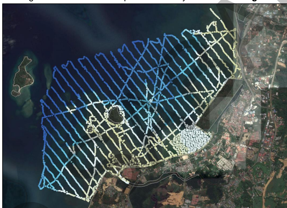
Figure 5.1(a): Bathymetrical survey at the Project site
